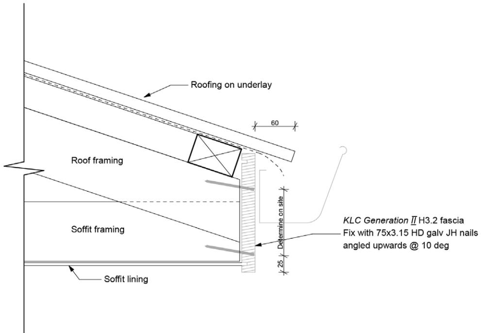
KLC Generation II H3.2 products have a premium factory applied alkyd primer and undercoat applied in two separate coats.
