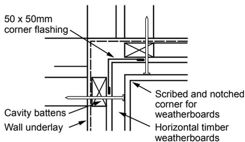
**(c) Cavity - Internal Butt Corner**
